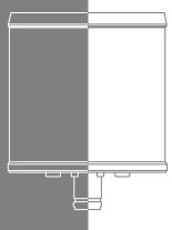
The LEDair 2 obstruction light is designed for marking aviation obstacles such as masts, chimneys, towers, cranes and buildings.
