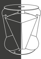
The radar reflector type SR6 is a passive radar reflector for use on buoys and beacons. Special features of this radar reflector are its 6-corner reflector plates in speckle design with optimised reflection properties.
